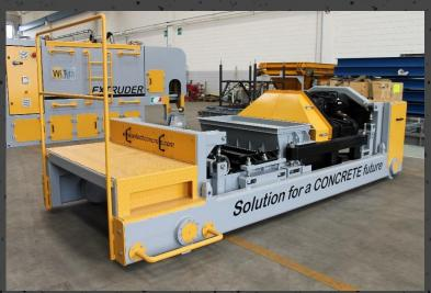
The machine is composed of two groups, a control and concrete feeding unit, called Silo, and a mechanical part dedicated to the proper hollow-core slab production, called Assembly.
