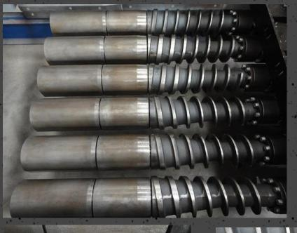
The Witech Extruder is made with a new technology, the machine doesn't use any internal vibrators for concrete compaction,
